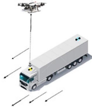
Fig. 8 UAV vehicle anchoring - step 2: Anchor and follow the vehicle
