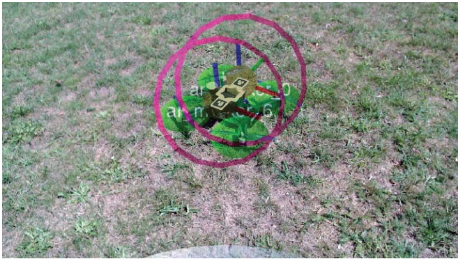
Fig. 11: The UAV is detected from the video feed of the arm's camera by means of the markers placed on the interface. The position of the markers is denoted by the two circles, while the orientation is shown through the superimposed coordinate frames. The virtual model of the UAV (shown in green) is also overlaid onto the live video stream.
