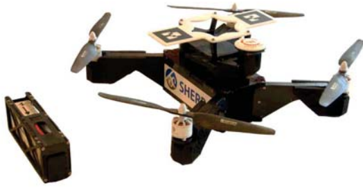
Fig. 3: The small scale UAV - the SHERPA wasp - and one of the exchangeable batteries
