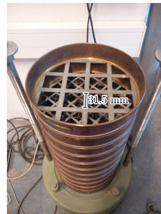
Fig. 4. Photograph of the multi-stage vibrating sieves used in this study.
