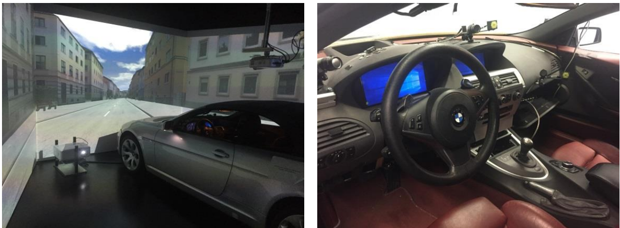
187 Figure 1. The TU Munich Driving Simulator. Left: full-vehicle mock-up; Right: cabin.
