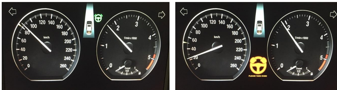
223 Figure 3. Photos of the instrument cluster with automation status. Left: automation available, corresponding to 224 Figure 2b; Right: take-over request, corresponding to Figure 2e.
