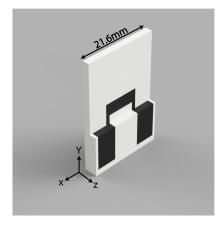
Fig. 1. 3D-model of the tactile sensor
