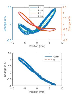
Fig. 5. Strongly reduced hysteresis due to differential measurement
