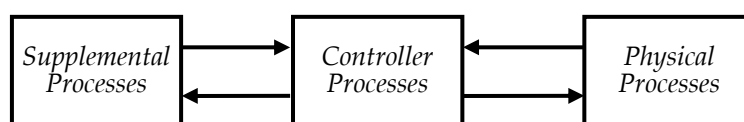
Figure 2-1 Context diagram (part 1 of 2) of a control system showing communication relationships between the controller, physical, and supplemental processes.
