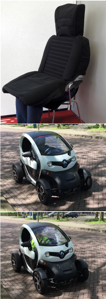
Figure 3: Top – the seat suit used for Wizard of Oz prototype for autonomous vehicles. Middle and bottom – The pedestrian’s view of one of the vehicles in autonomous and manual mode respectively
