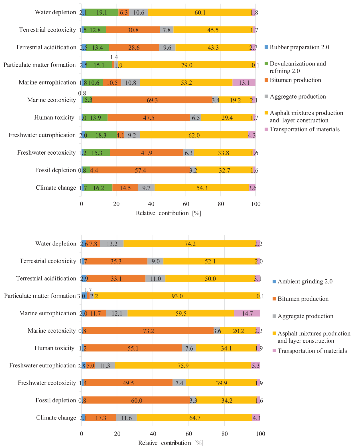
Figure 4. Relative contribution of the different life cycle phases and subphases for the total environmental impacts due to the use of (a) asphalt mixture with 2.0% of vulcanised CR and (b) asphalt mixture with 2.0% of devulcanised CR.
