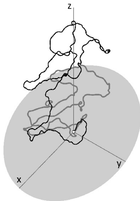
Fig. 4. Scheme of the random conformational polymer chain (black) and adsorbed polymer chain (gray) at the surface of the substrate.
