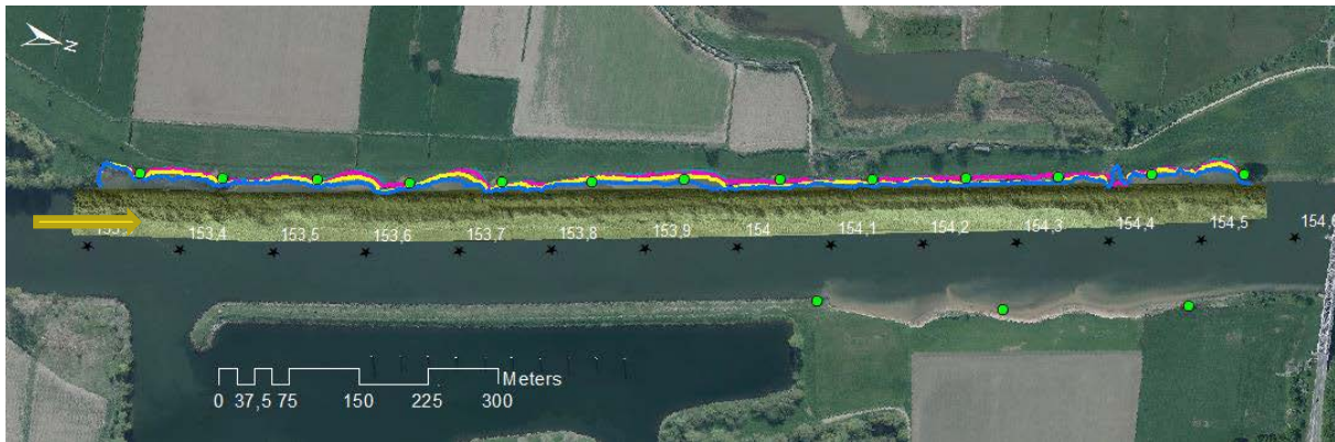
Figure 2. Bank lines in the Maas over four years of naturally eroding conditions (blue 2011, yellow 2012, pink 2013, green 2014).
