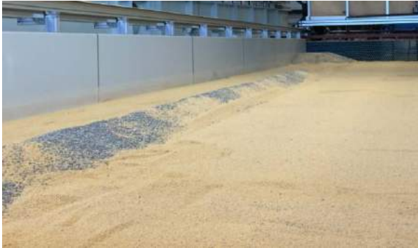
Figure 3. Scale model of the upstream section of a longitudinal training dam (1:60) in a 2.5-metre-wide flume in the Kraijenhoff van de Leur Laboratory for Water and Sediment Dynamics in Wageningen.
