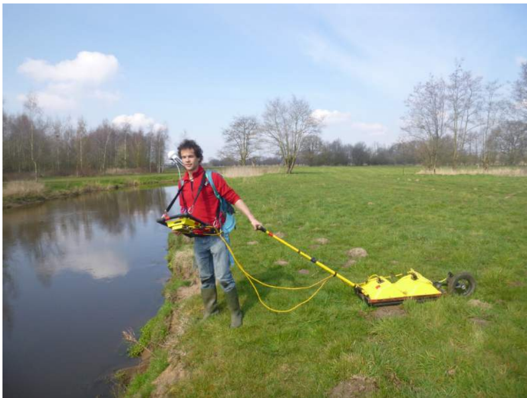
Figure 1. Using ground-penetrating radar (GPR) to study the fluvial deposits in the Dommel valley.
