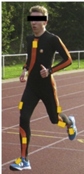
Fig. 1. Measurement set-up. IMUs are visualized at the feet, medio-anterior part of the tibia, upper legs lateral at the iliotibial tract and sternum (the manubrium). Note that the IMU at the sacrum is not visible.
