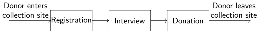
Figure 5.2 Schematic model of a collection site. Every station is modeled as a M/M/s queue.
