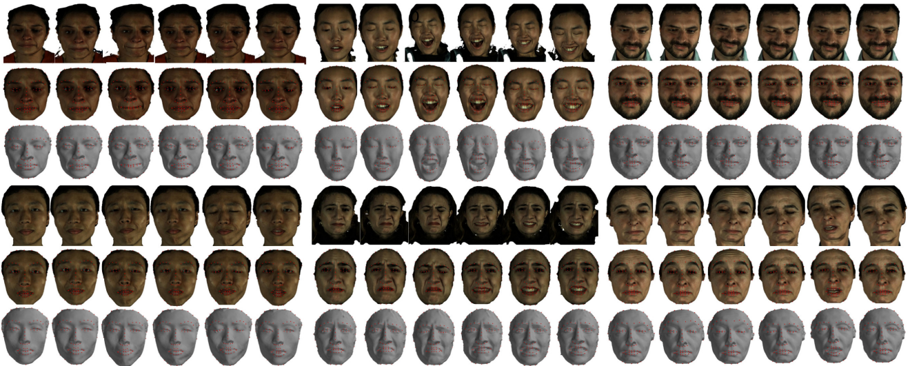
Figure 4: 4D sequences that are in full correspondence with template, displayed with 79 landmarks. For each sequence, top row shows original scans, middle and bottom rows are the registered 3D meshes with and without texture respectively.
