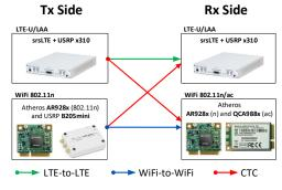
Fig. 9. Platforms used for LTE\*-WiFi prototype.
