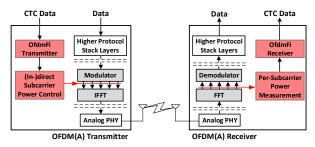
Fig. 4. The conceptual architecture of OfdmFi with colored blocks showing the required OFDM technologies' extensions.
