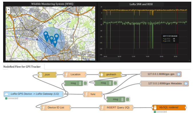
Fig. 4: WMS location tracking application on the LoRa server, a map showing near Univ. Twente Campus
