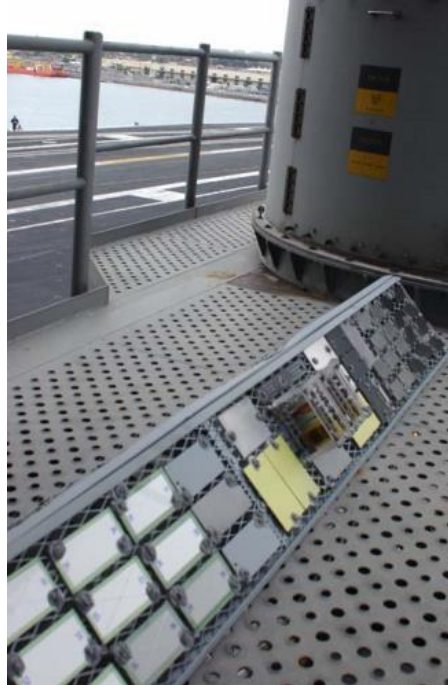
FIGURE 1. SPECIMENS FITTED ON EXPOSURE RACK ON DECK OF THE USN CVN 74 (NIMITZ-CLASS NUCLEAR-POWERED SUPERCARRIER) TO PERFORM CORROSION RATE ASSESSMENT OF THE MARITIME ENVIRONMENT 123 .
