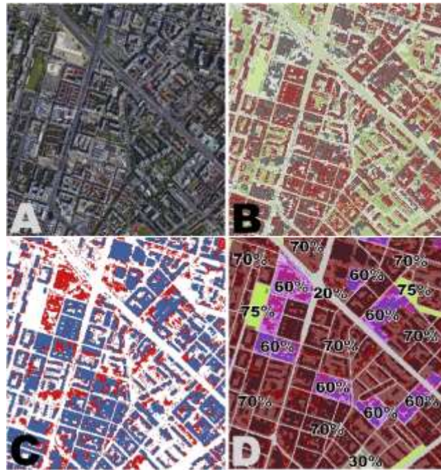
Figure 88 (A) Aerial photo (B) Overlay of ESM (grey patches) and cadaster data (red polygons). (C) Observed overshoot in the ESM (red patches) to be filtered out. (D) Calculated scaling factors per land cover class. Source: [2]
