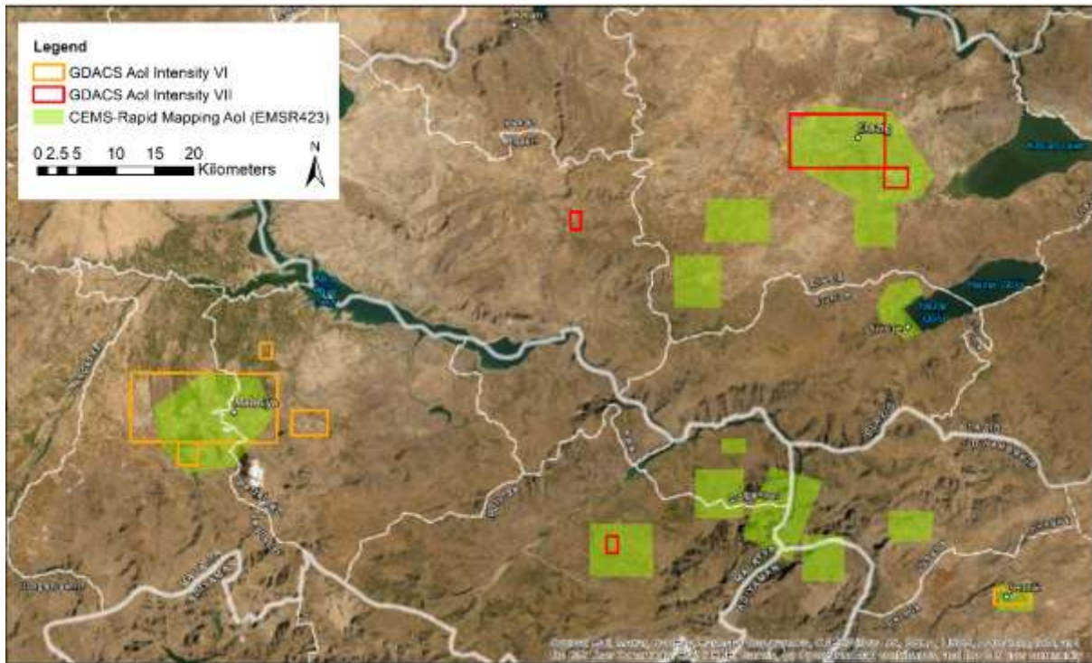
Figure 35 Earthquake in Turkey 24 January 2020: comparison of Aols generated by GDACS and the areas which were analysed under CEMS-Rapid Mapping for actual impact using satellite images. The satellite-based impact assessment confirmed damages in the GDACS Aols of the highest intensity class.
