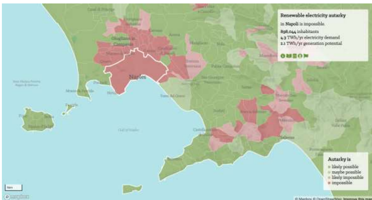
Figure 87 Screenshot of the interactive map visualising the main results of our study. The map visualises the potentials for each of the 34 countries, 502 regions, and 122,635 municipalities. Municipalities coloured light green and light red may be able to achieve renewable electricity autarky by allowing for higher local densities of electricity infrastructure. Available at: https://timtroendle.github.io/possibility-for-electricity-autarky-map/
