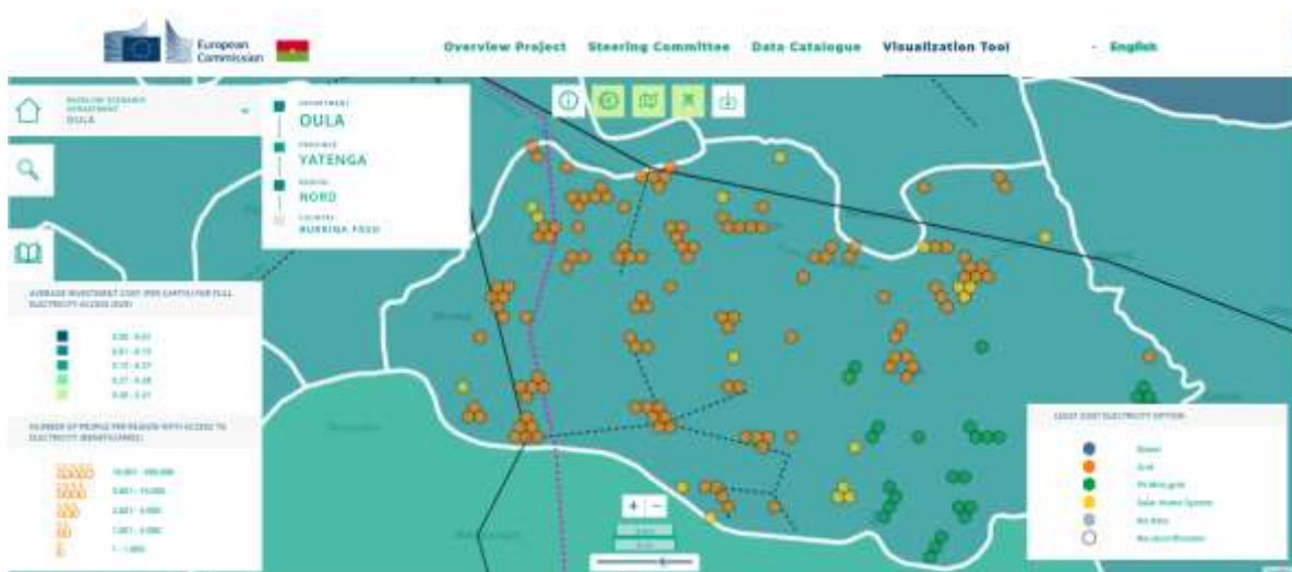
Figure 62. OPER-BU least-cost option per settlement (grid extension, diesel generator, PV mini-grid or PV stand-alone system)
