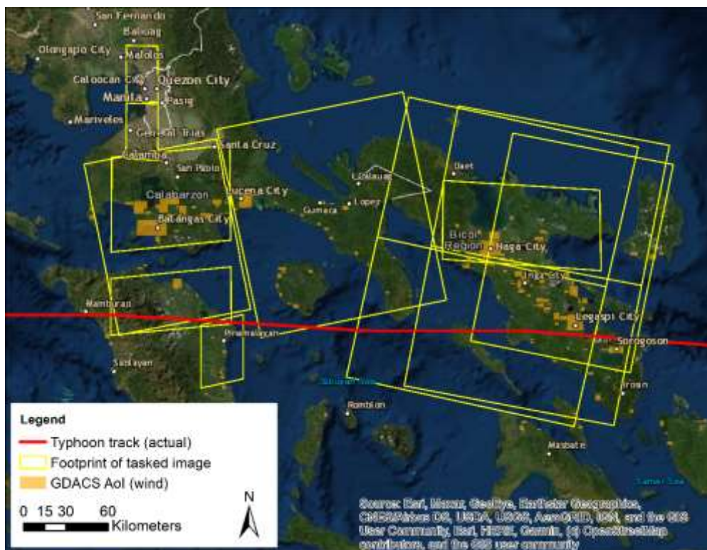
Figure 36 Typhoon Kammuri December 2019: comparison of Aols generated by GDACS (wind impact), actual storm track and the footprint of pro-actively tasked satellite images.
