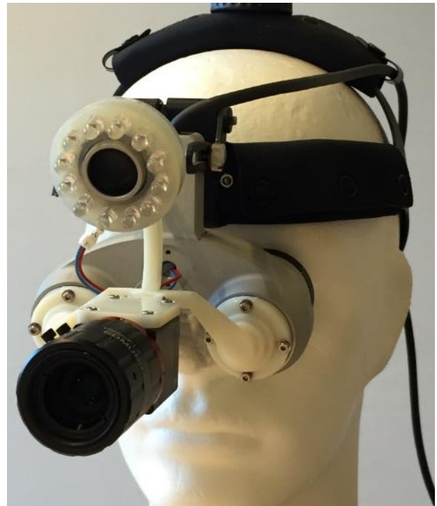
Fig. 4. Demonstrator of H3D-VISIO n AiR. Spectral+RGB camera, head mounted display, dedicated infrared LED ring.
