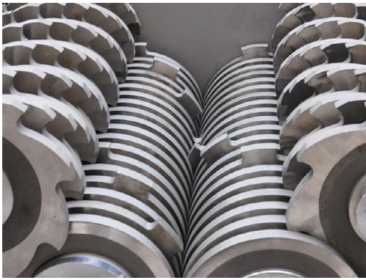
Fig. 3. Inside view of a four-shaft shredder (image courtesy of UNTHA GmbH).
