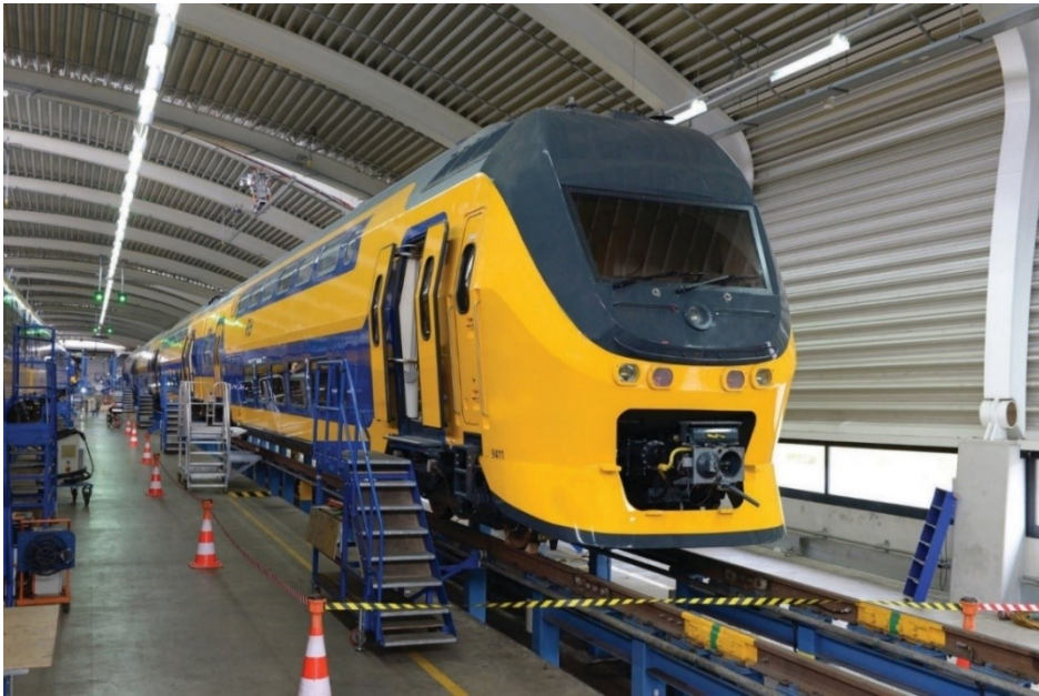
Figure 6.6: VIRMm1 train during modernization at NSTM, extending its life another 18 years.
