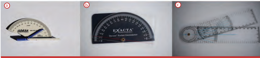
Figure 3.3 Goniometers used in this study: (a) Rolyan finger goniometer with loose-fitting hinge; (b) Devore pocket goniometer; and (c) universal goniometer with full-circle body.
