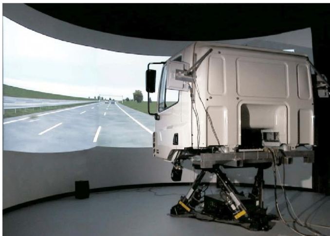
Figure 3.1: TNO truck driving simulator with moving hexapod and cylindrical projection screen
