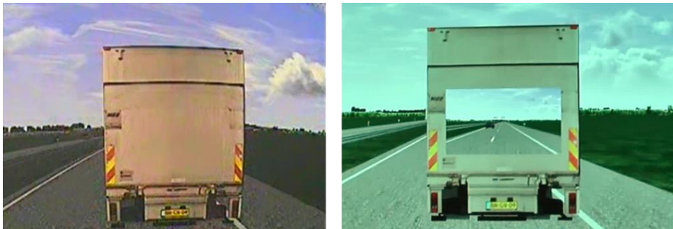
Figure 6.1: Screenshot of a normal lead truck (left) and a see-through lead truck (right) in the simulation
