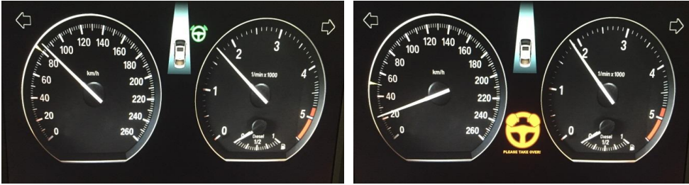
Figure 7.3: Photos of the instrument cluster with automation status. Left: automation available, corresponding to Figure 7.2 b; Right: take-over request, corresponding to Figure 7.2 e.
