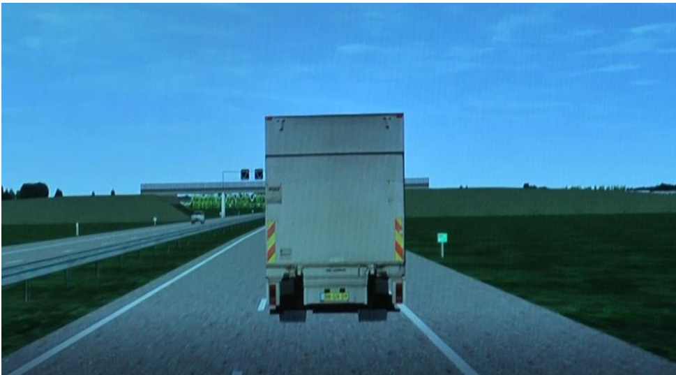
Figure 3.3: Front view in the second truck. The center of the ego lane was blocked by the lead truck, while the driver was able to perceive traffic information from the adjacent lanes
