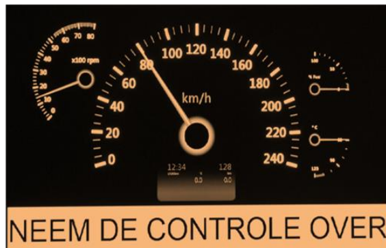
Figure 3.4: Visual interface of the take-over request (text in Dutch: “Take over control”)
