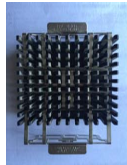
Heat sink: Without it, a CPU will burn out. Unfortunately, I don't have a picture of MY heat sink.
