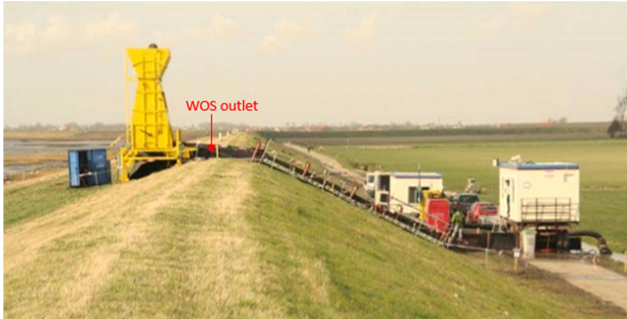
Fig. 4 Overview of the test set-up of the hydraulic measurements (from Dutch Ministry of Infrastructure and the Environment 2012). The measurements will be used to validate the hydrodynamic conditions at the simulator outlet of the hydrodynamic model
