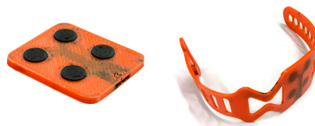
Fig. 1. Photograph of 3D-Printed electrodes using flexible conductive filaments.
