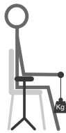
Fig. 3. Position of the subject performing the load experiment. The elbow is placed on an arm rest, the load is increased from 0 kg to 5 kg over 10 seconds.
