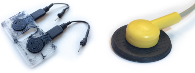
Fig. 2. Left: 3D-printed electrode after assembly. Right: Connected printed electrode used for patient ground.
