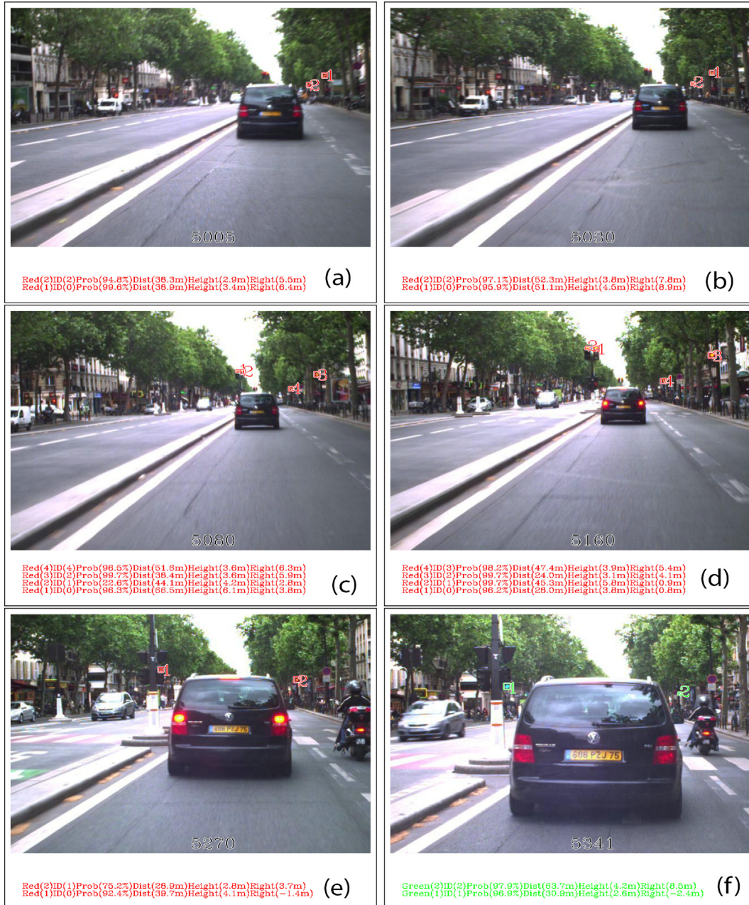
Fig. 8. The traffic lights are detected in LARA dataset (a) from beginning, (b) after 1 s, (c) after 3 s, (d) after 6 s, (e) after 11 s, (f) after 14 s. The signals are correctly recognized and the position of the traffic lights is estimated with respect to the camera.
