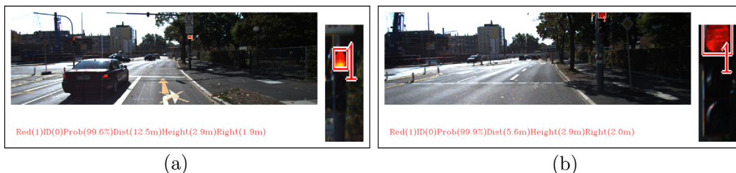
Fig. 4. The traffic light detection for the KITTI dataset; (a) The lower part of the red signal has more illumination and it is transformed to yellow. Therefore, the color of the signal should be evaluated for every pixel and the choice of the color should be estimated in a voting scheme. (b) The traffic light is partially occluded, but the algorithm can detect the traffic light since it imposes the temporal consistency constraint. (For interpretation of the references to color in this figure legend, the reader is referred to the web version of this article.)
