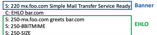
Figure 2: Banner and EHLO message in a typical SMTP session between client (C) and server (S).
