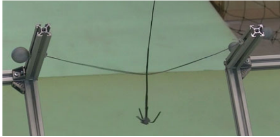
Fig. 6.2 Zoom of the hook and the anchoring mechanism
