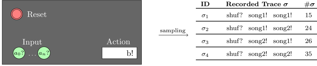
Fig. 5. Black box trace machine with input alphabet a_0?, \dots, a_n? , reset button and action window. Running the machine m times and observing traces of length k yields a sample. The ID together with the trace and the respective number of occurrences are noted down
