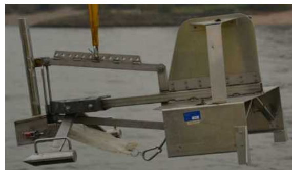
Figure 1. Improved Arnhem Sampler, as used by the German authorities (top) and Delft Nile Sampler, as used by the Dutch authorities (bottom). Note the difference in mesh size and the sample container.
