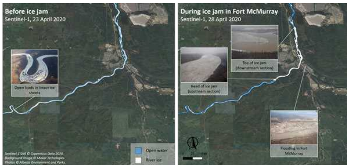
Figure 1: River ice jam flooding in Fort McMurray, Canada as seen from Sentinel-1 and dedicated aerial surveys. Contains modified Copernicus Sentinel data [2020]. Background image © Maxar Technologies. Photos © Alberta Environment and Parks.
