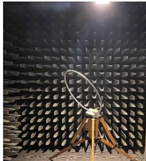
Fig. 5. Transmitting antenna position tilted to 45 degrees in X , Y , and Z axis.
