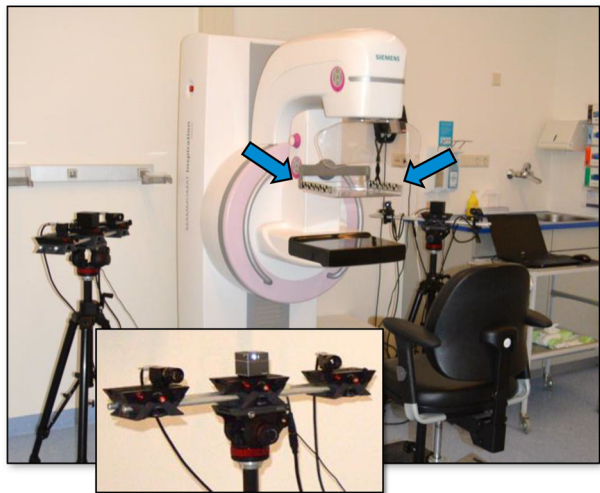
FIGURE 1 SL scanning system setup: one projector with two cameras is placed on each side of the DBT system (see close-up image) and markers were added to the compression paddle to ensure good alignment in the post-processing step (top blue arrows). DBT, digital breast tomosynthesis; SL, structured light.
