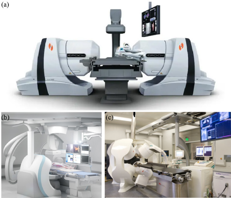
Figure 1.4: Commercially available magnetic actuation systems: (a) Stereotaxis Niobe Robotic Magnetic Navigation System [41] (b) Aeon Phocus, interventional robotic system [42] (c) Catheter Guidance Control and Imaging (CGCI) system [43]
