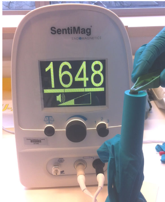
Figure 1 Selection of lymph nodes with uptake of magnetic tracer. A blue formalin-fixed lymph node is placed on the handheld probe (covered with a surgical glove) of the magnetometer with plastic tweezers. The numerical display of the system is used to quantify the uptake of magnetic tracer.
