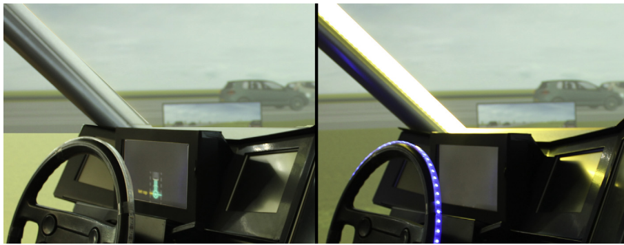
Fig. 7. Pictures showing concept B (left) and concept C (right) during the hazard alert for an approaching vehicle in a highway-merge situation. Concept B depicts an icon behind the steering wheel, and concept C uses illumination of the pillar aside the windscreen. Both alerts were only visual.
