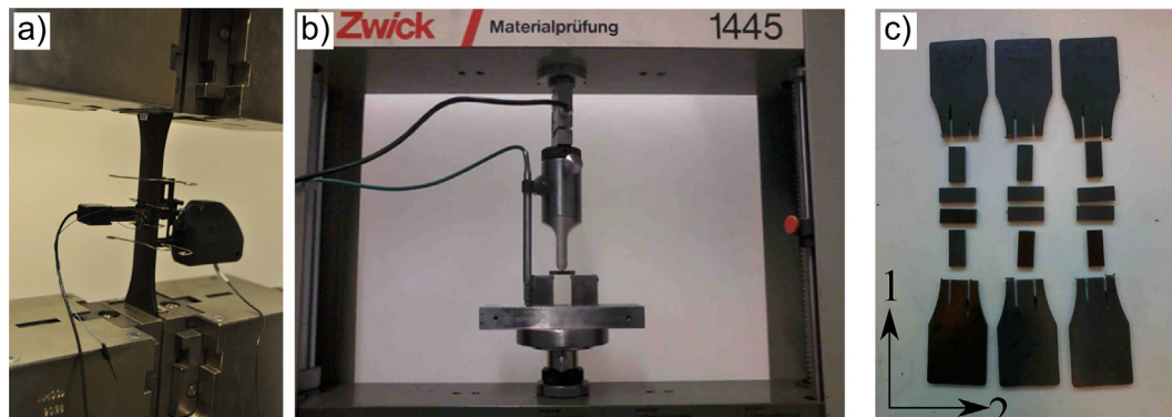
Fig. 2. (a) Set-up used for the measurement of tensile properties of the filler. (b) Set-up used for the measurement of bending properties of the filler. (c) Short beam specimens for longitudinal and transverse properties. Fibers are oriented in the 1-direction.
