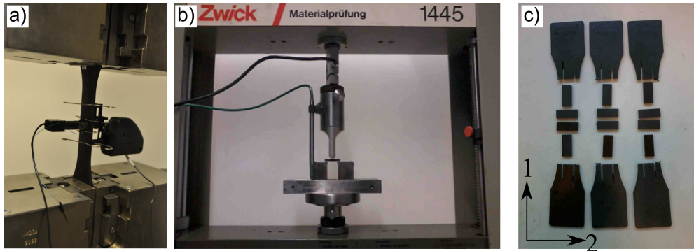
Figure 2: a) Set-up used for the measurement of tensile properties of the filler. b) Set-up used for the measurement of bending properties of the filler. c) Short beam specimens for longitudinal and transverse properties. Fibers are oriented in the 1-direction.
