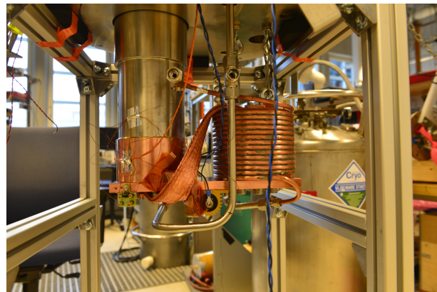
(b) A picture of the inside of the cooling box, containing the cooler, thermal link and heat exchanger.
