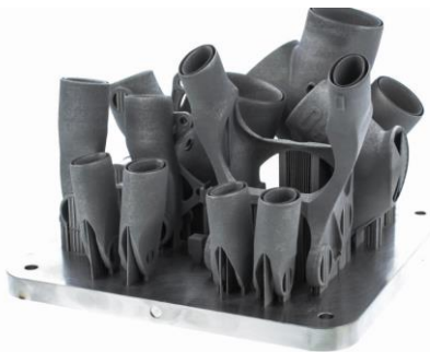
Figure 28.4. Titanium lugs with build plate, produced by additive manufacturing (Renishaw, 2016)
