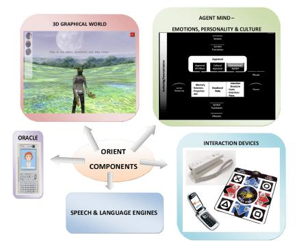
Figure 1: ORIENT system components
