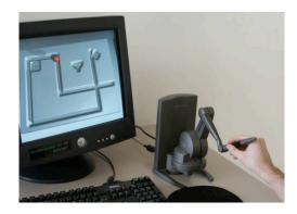
Fig 1: PHANToM® desktop and visualized VETM
