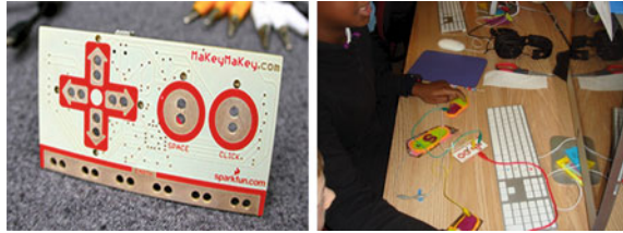
Fig. 2 The MaKey MaKey board ( left ) and a hooked up version ( right )
