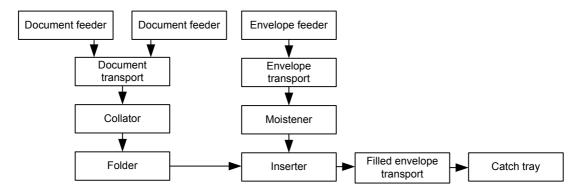
Figure 10: Diagram of the mechanical plant parts and path of paper and envelopes
