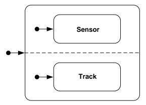
Figure 1-12: Parallel state machines describing movement along the sensor and track. The sensor stays On for the number of pulses that correspond to the paper length. The track stays occupied for the number of pulses that correspond to the track length.
