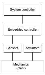
Figure 9: The system architecture
