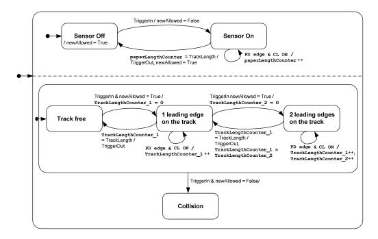
Figure 1-16: The track state machine describing a long track- it can contain two leading edges of two separate papers. In the state '2 leading edges on the track', two leading edges are present. As soon as the first one leaves the track, counter 1 should have the value of counter 2 as it will continue to track the second leading edge that will become the first leading edge in the track.
