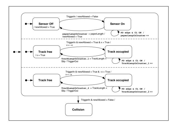
Figure 1-17: Two parallel state machines describe movement of two pieces of paper on a long track. Sensor
