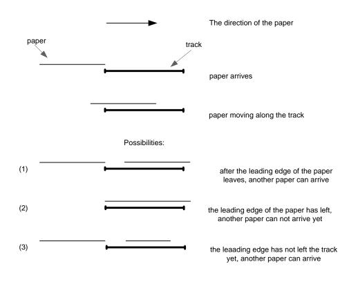
**Figure 1-18: Different possible lengths of a track**
