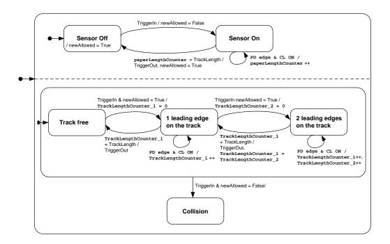
Figure 1-20: The track state machine describing a track that can have two leading edges of two separate papers present at the same time. In the state '2 leading edges on the track', two leading edges are present. As soon as the first one leaves the track, counter 1 should have the value of counter 2 as it will continue to track the second leading edge that will become the first leading edge in the track.
