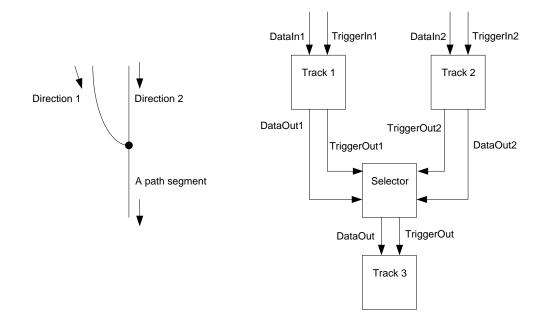
Figure 1-22: Left side: sketch of the two paths joining together. Right side: their representation in the model, where selector forwards the data about the material that arrived.
