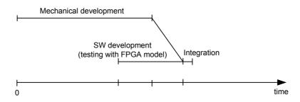
Figure 7: The timeline of development and the integration, when the emulator is used.
