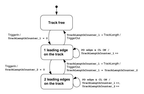
Figure 1-15: State machine describing a long track
