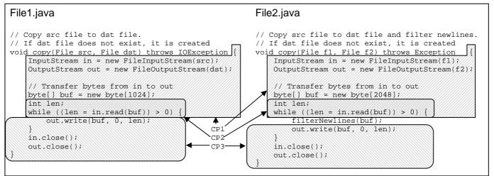
Figure 1 Clone pairs CP1, CP2 and CP3 detected according to different rules and definitions
