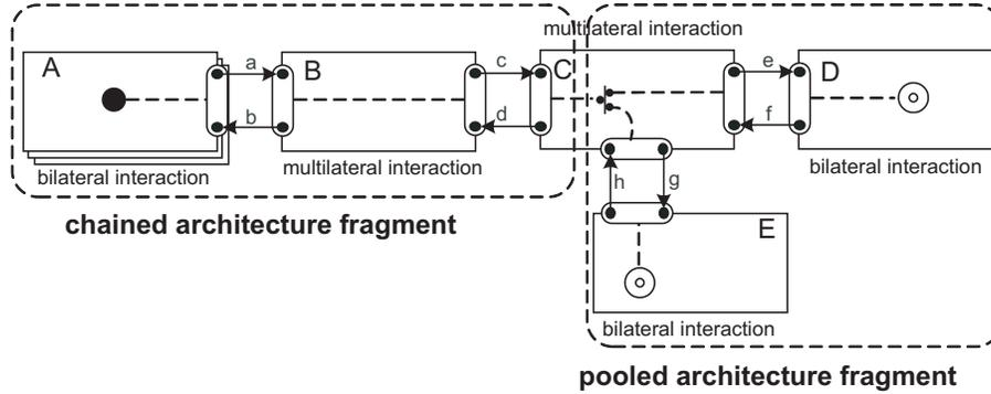
**Fig. 5.** Decomposing a value web into two architectural fragments.
