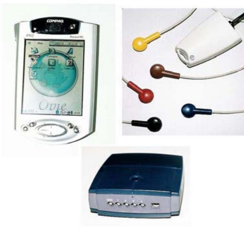
Fig. 3b. One BAN configuration: PDA, front-end and sensors
