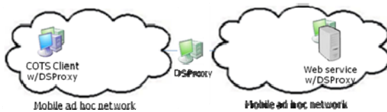
Figure 1: A simple network layout showing two discrete networks bridged with a DSProxy, adding store-and-forward capability to a standard Web service.
