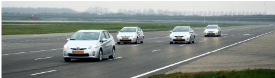
Fig. 1. Four CACC operated vehicles during practical testing.
