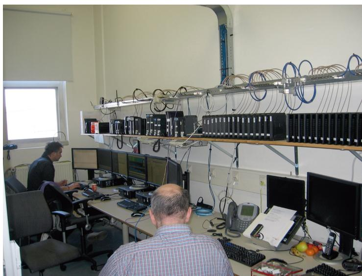
Laboratory for testing cable modems
