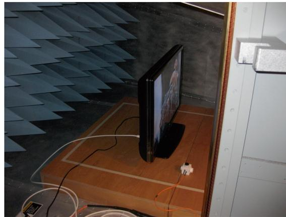
Figure 4 and 5. Sensor near set-top box and television set in GTEM
