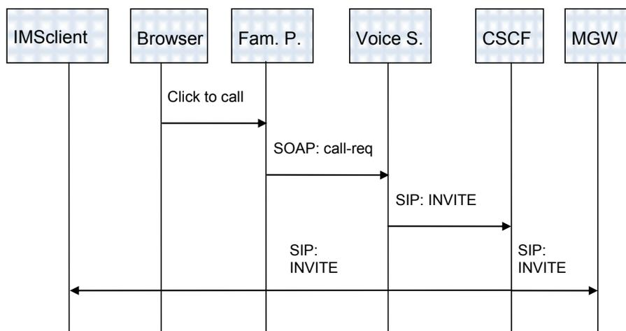
**Figure 4 Sequence diagram of making a call**
