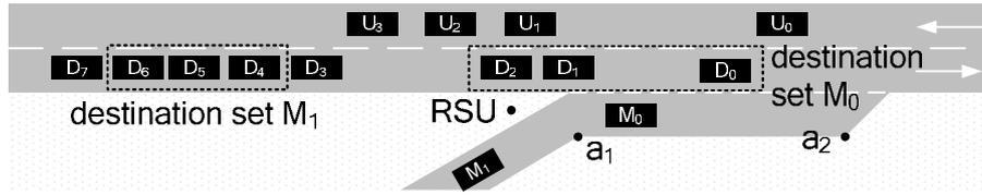
**Fig. 1.** Merging vehicles wish to join the downstream freeway vehicles. The arrows denote the direction of travel. The dotted lines represent the borders of geocast destination sets. The subnetworks of downstream travelling vehicles are  $D_0, D_1, D_2,$  and  $D_3$ - $D_7$ .
