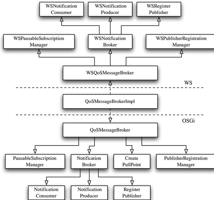
**Fig. 3.** Web Service and OSGi interface of the QoS message broker
