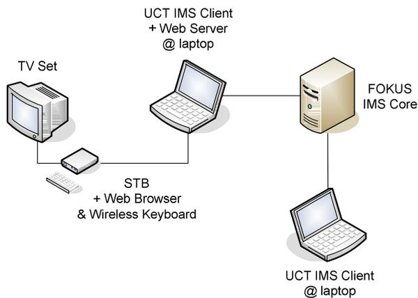
**Figure 5 The Mobicome IMS-IPTV testbed**
