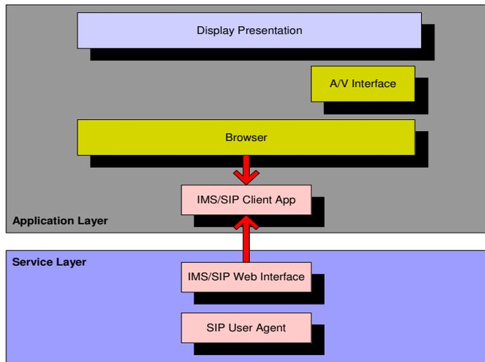
**Figure 3 Functional architecture of the Mobicome IPTV CND**
