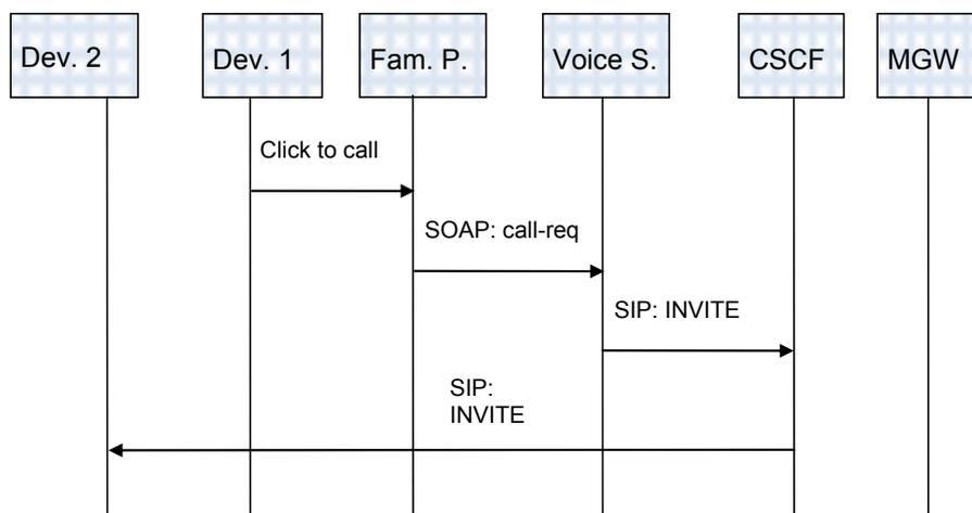
**Figure 5 Sequence diagram of call transfer between devices**
