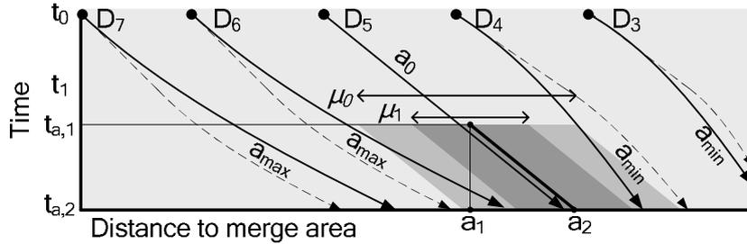
**Fig. 2.** The trajectories of five freeway vehicles of Fig. 1 through time and space. The merger's trajectory has also been projected on the figure as a line between the points  $(t_{a,1}, a_1)$  and  $(t_{a,2}, a_2)$ . The shaded parallelograms represent the margin  $\mu$  around the merging vehicle during  $[t_{a,1}, t_{a,2}]$ , calculated at  $t_0$  and  $t_1$ . The dotted trajectory for  $D_5$  is hidden beneath the solid trajectory.
