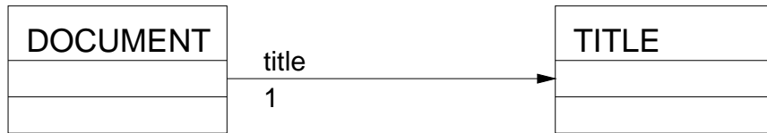
Figure 6.5: There is exactly one document for each title, and there is exactly one title for each document.
